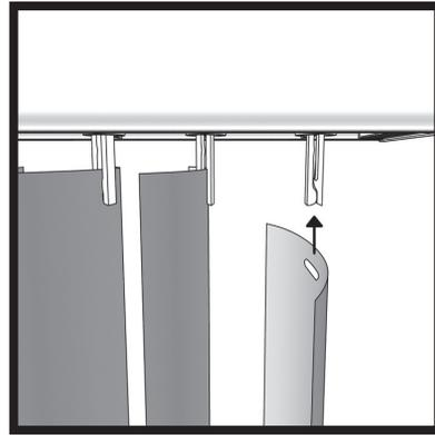
**NOTE:** All the tracks are reversible depending on which side you would like to locate your stacking and controls. Make sure to leave a 2" space between the installation screw on the release flange and the wall/window or any protruding handle or window frame.
